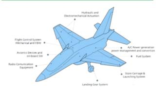
Hydraulic & electromech. actuation Electric power generation Electric power management Flight Control System Radio communication equipment Avionics & Navigation Landing gear system Storage carriage & launching Ground support equipment Structures & Materials Components
