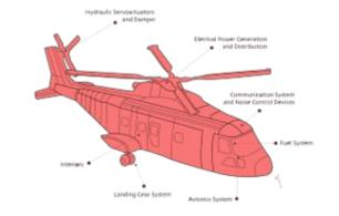
Hydraulic servoactutors & Dampers Electric power generation Electric power management Radio communication equipment Vibration reduction systems Interiors Noise reduction systems Avionics & Navigation Landing gear systems Structures & Materials Components
